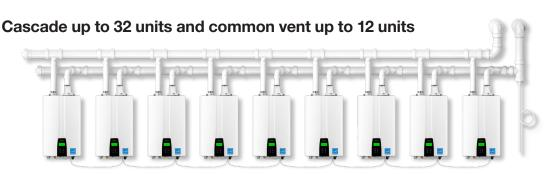
With Navien cascading technology, when a unit gets up to 80% capacity the next unit will turn on to help meet requirements. This demand ratio will continue until all 32 units are generating hot water. The Navien cascading system also balances out the workload of each unit for longer life. Building penetrations are reduced with Navien's common venting feature.
